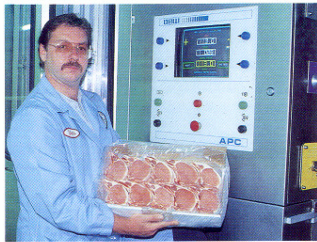
Operations director Stan Tokarz holds a box of portion control pork chops, cut to exact weight by the APC behind him.
