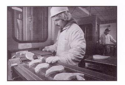
Technologies currently utilized at the plant include Automatic Portion Control systems, which can cut up to 180 portions per minute at plus or minus two grams to size; two injector machines are available to enhance their pork products with a solution to prevent the product from drying out when it is over cooked; and automatic pop-up timers are inserted into products to alert cooks when they are done.
